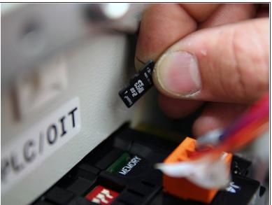
Remove microSD card from PLC by pushing down on card.
